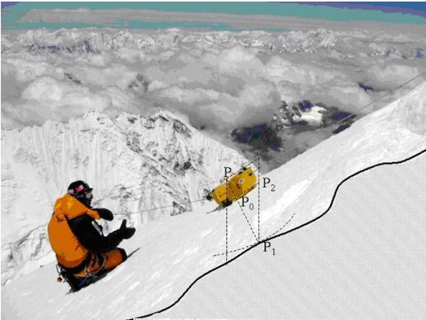
Fig. 6- Climber operating the GPR on the steep slope along the South West ridge.
